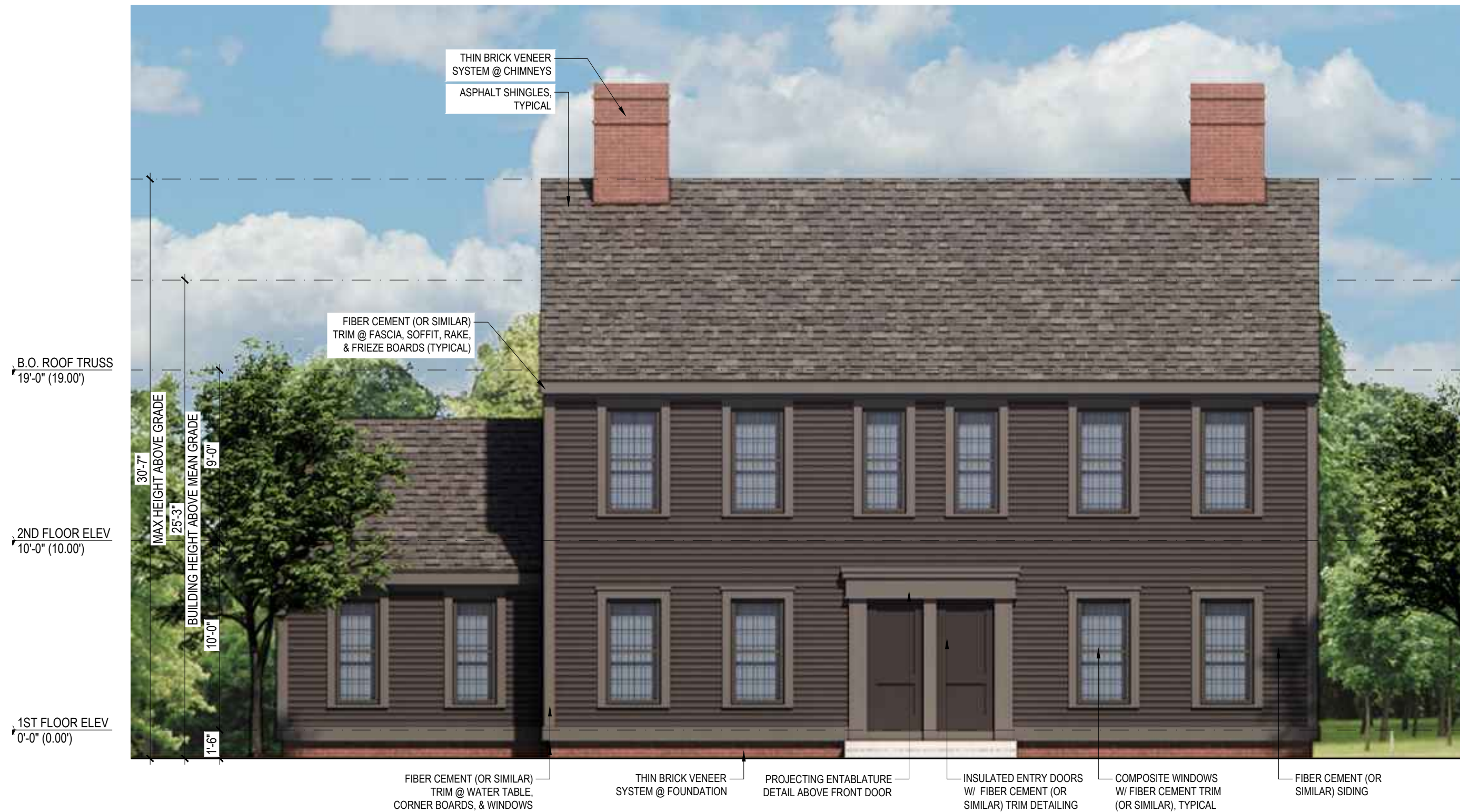
1 BUILDING B - NORTH-WEST ELEVATION SCALE: 3/16" = 1'-0"
