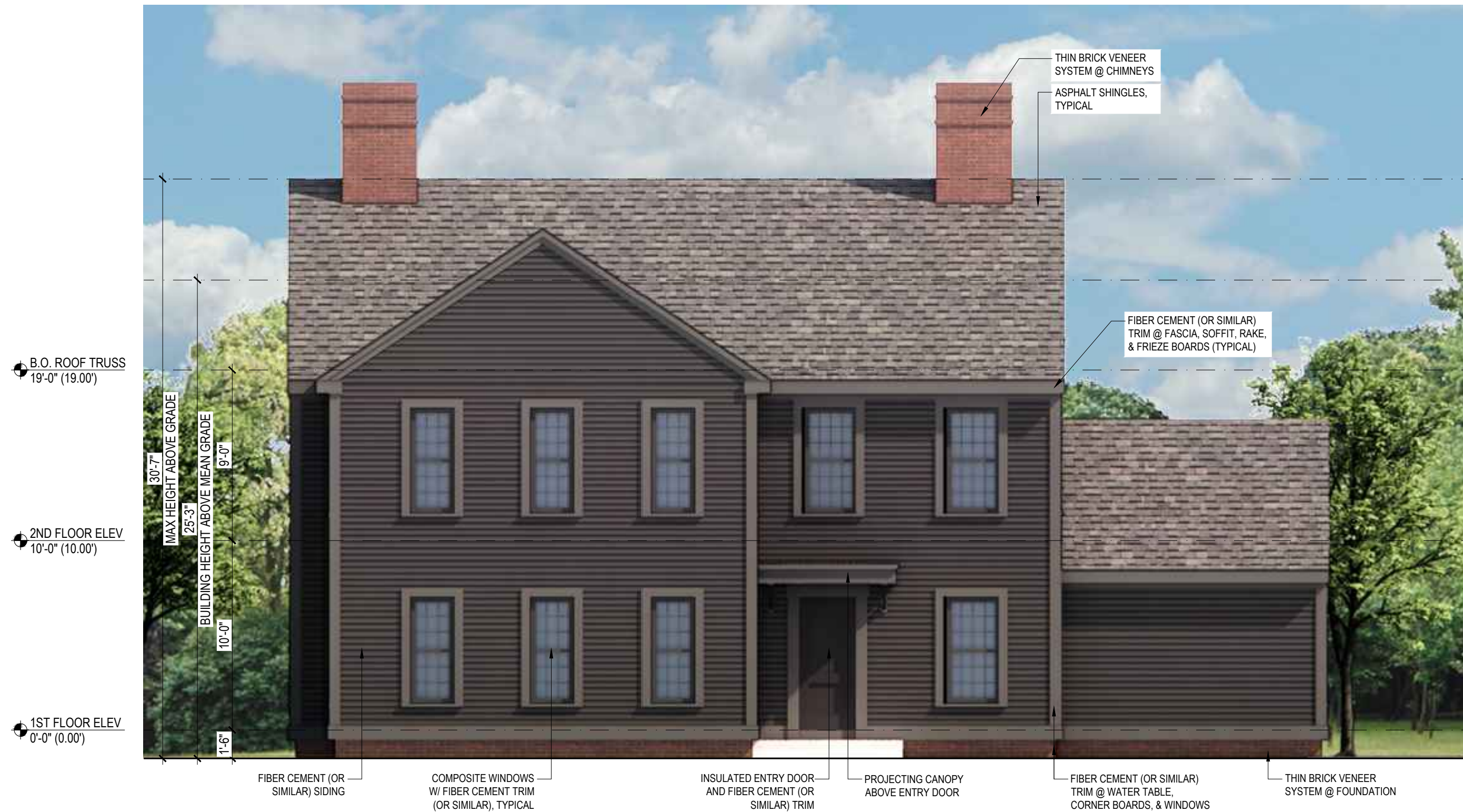
2 BUILDING B - SOUTH-EAST ELEVATION SCALE: 3/16" = 1'-0"
