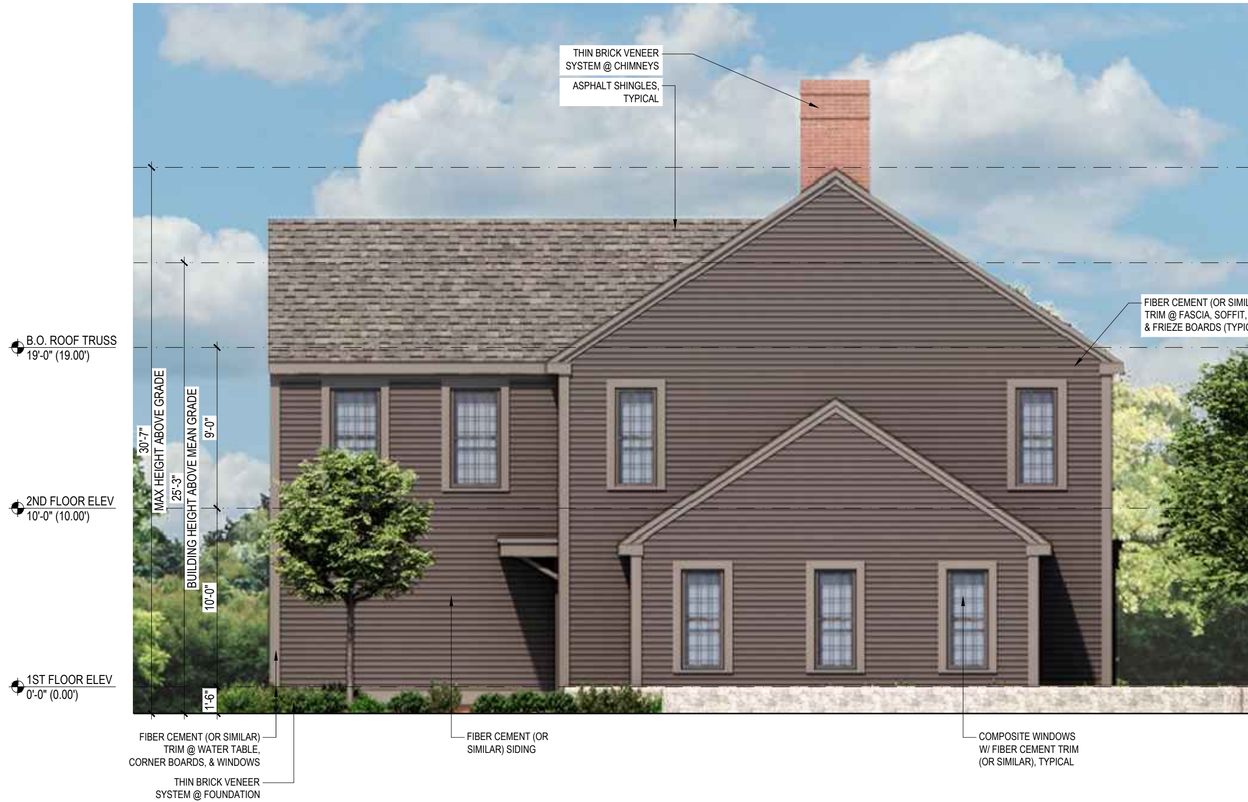
3 BUILDING B - NORTH-EAST ELEVATION SCALE: 3/16" = 1'-0"
