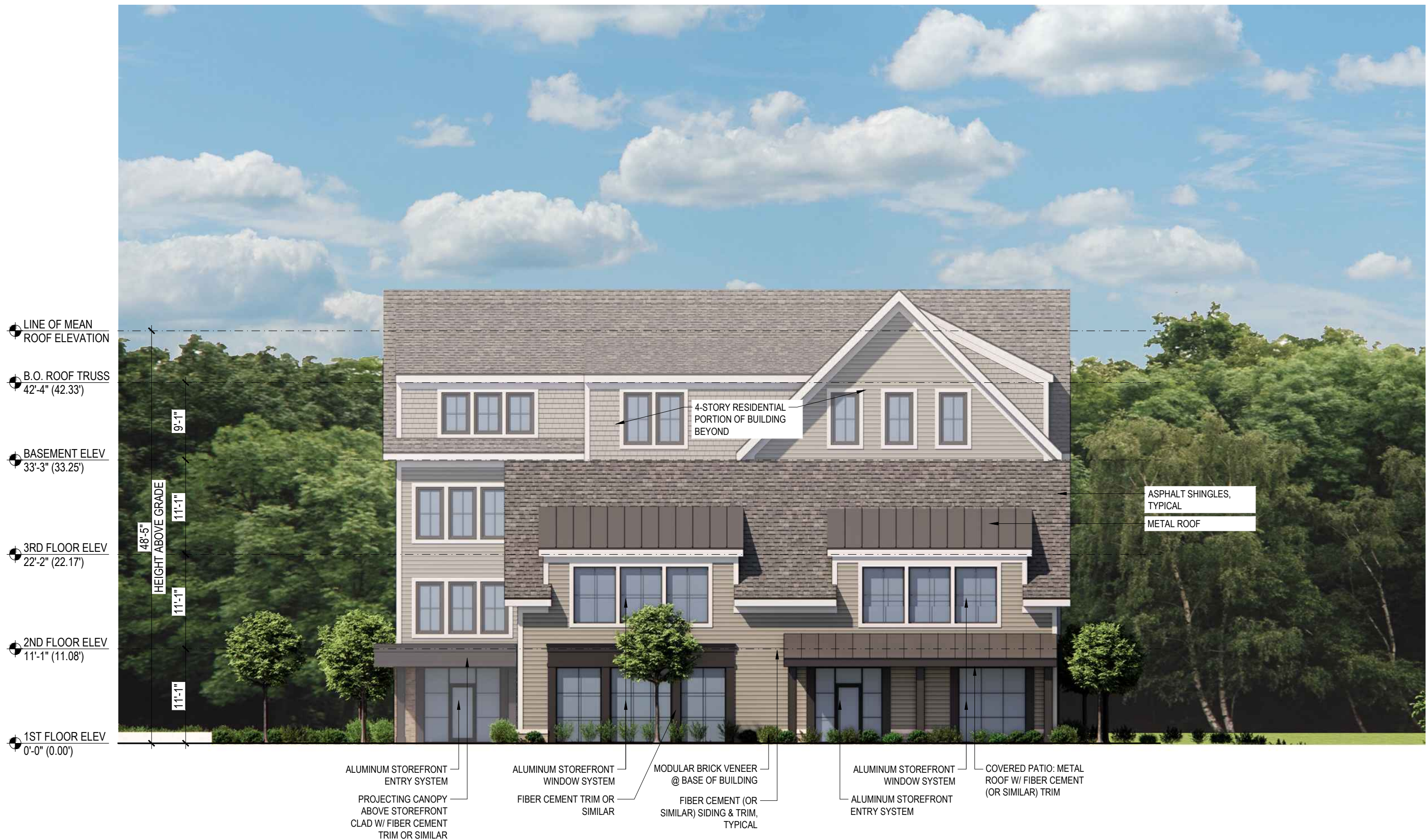
1 BUILDING C1 - NORTH-WEST ELEVATION SCALE: 3/32" = 1'-0"
