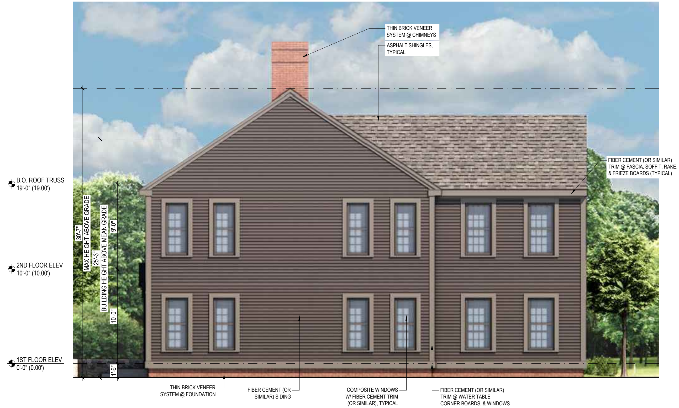
4 BUILDING B - SOUTH-WEST ELEVATION SCALE: 3/16" = 1'-0"
