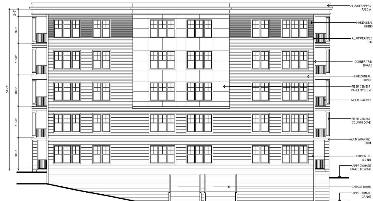
63 UNIT BUILDING - RIGHT SIDE ELEVATION
