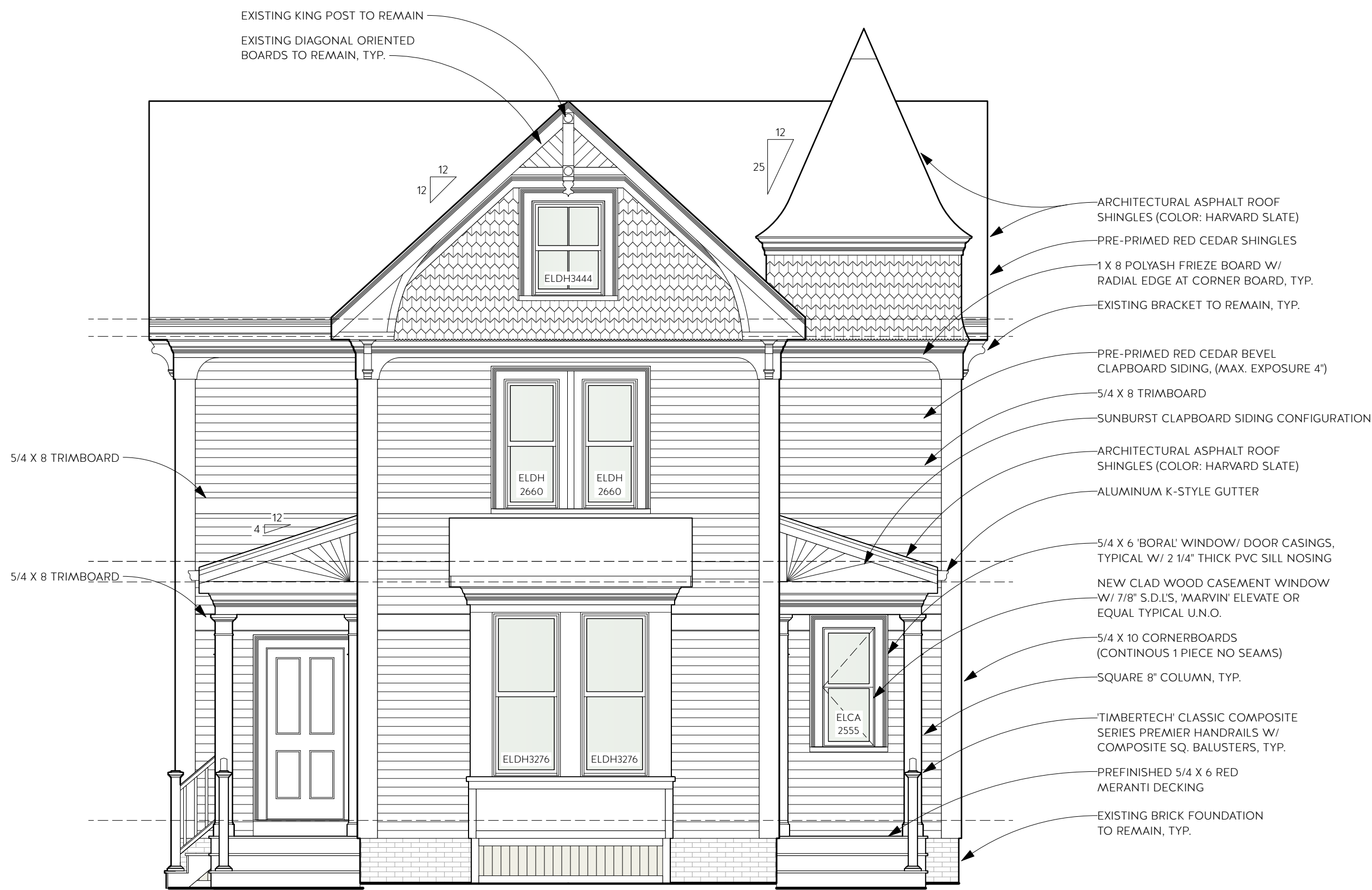
1 PROPOSED NORTH EAST (FRONT) ELEVATION Scale: 1/4" = 1'-0"
