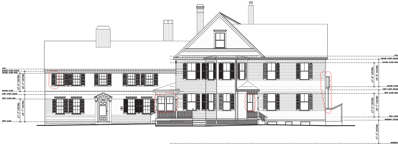
BUILDING D EXISTING RIGHT ELEVATION SCALE: 3/16" = 1'-0"
