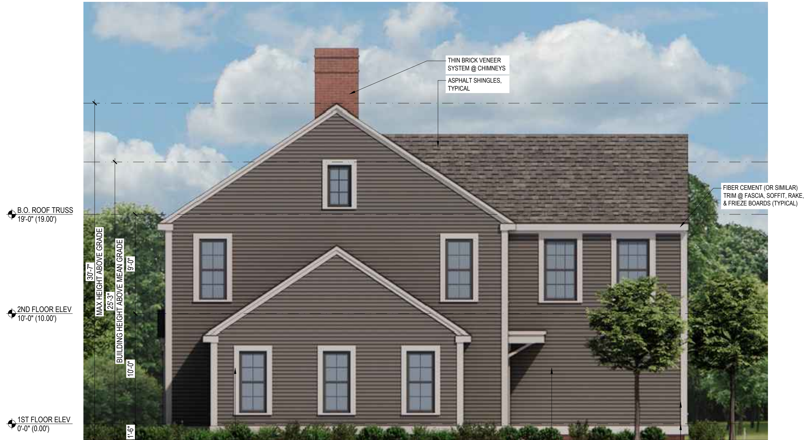
4 BUILDING A - SOUTH-WEST ELEVATION SCALE: 3/16" = 1'-0"
