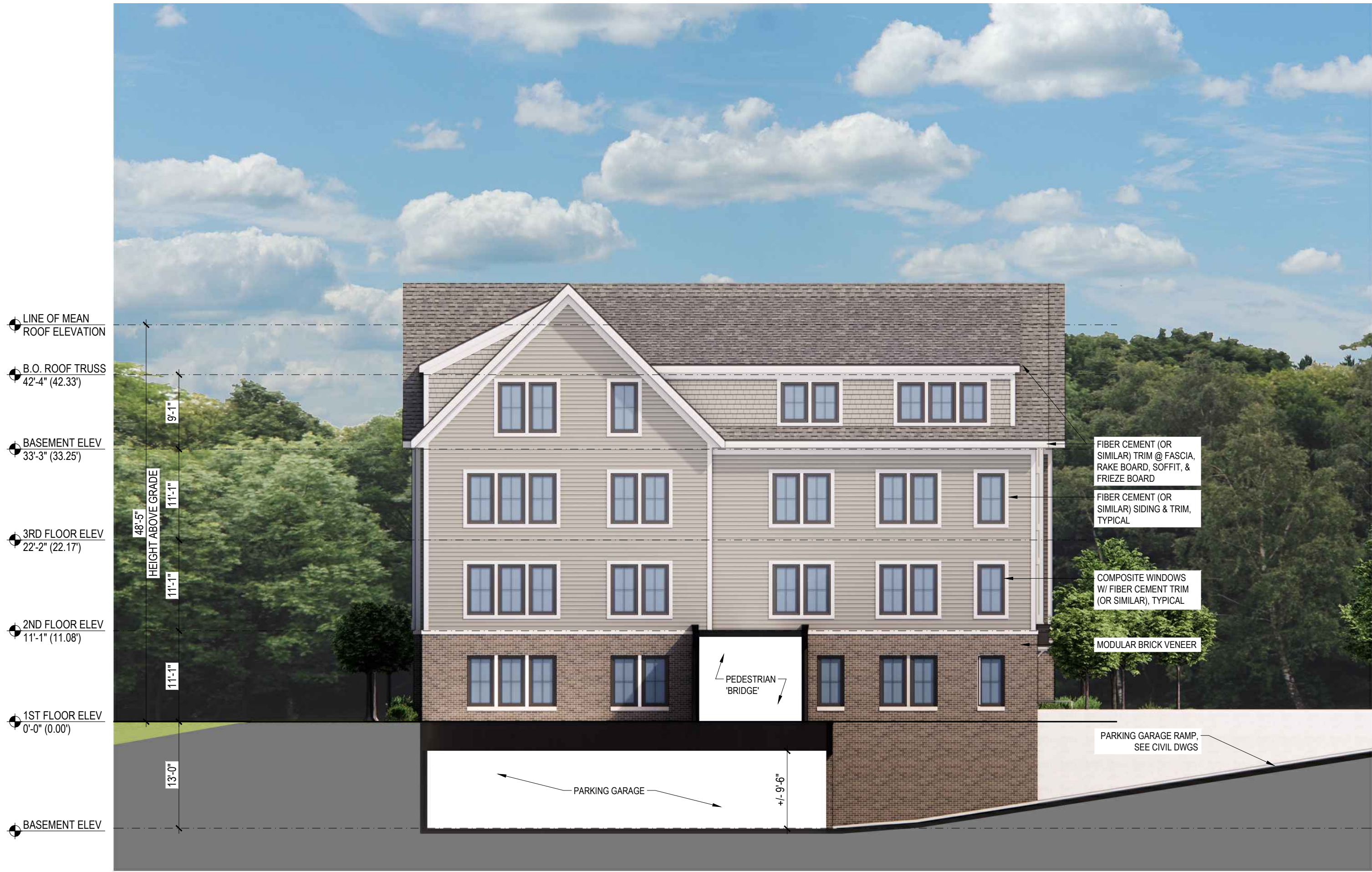
2 BUILDING C1 - SOUTH-EAST ELEVATION SCALE: 3/32" = 1'-0"
