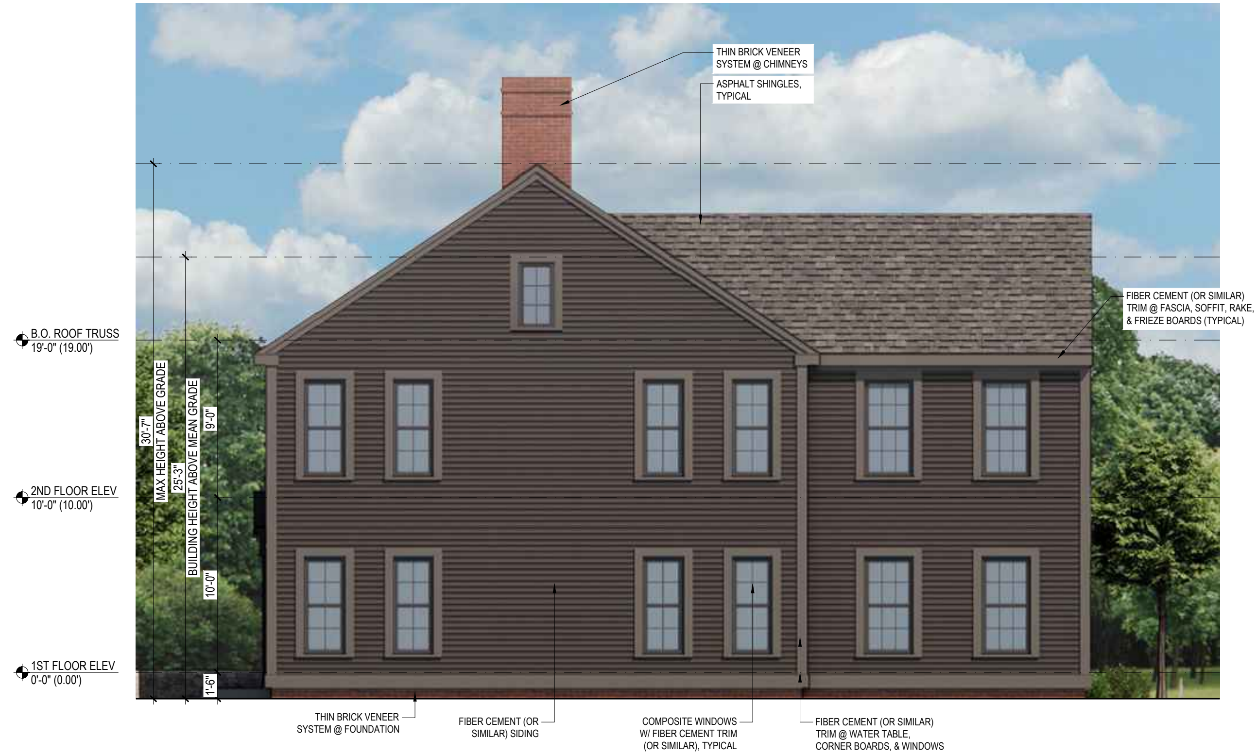
4 BUILDING B - SOUTH-WEST ELEVATION SCALE: 3/16" = 1'-0"
