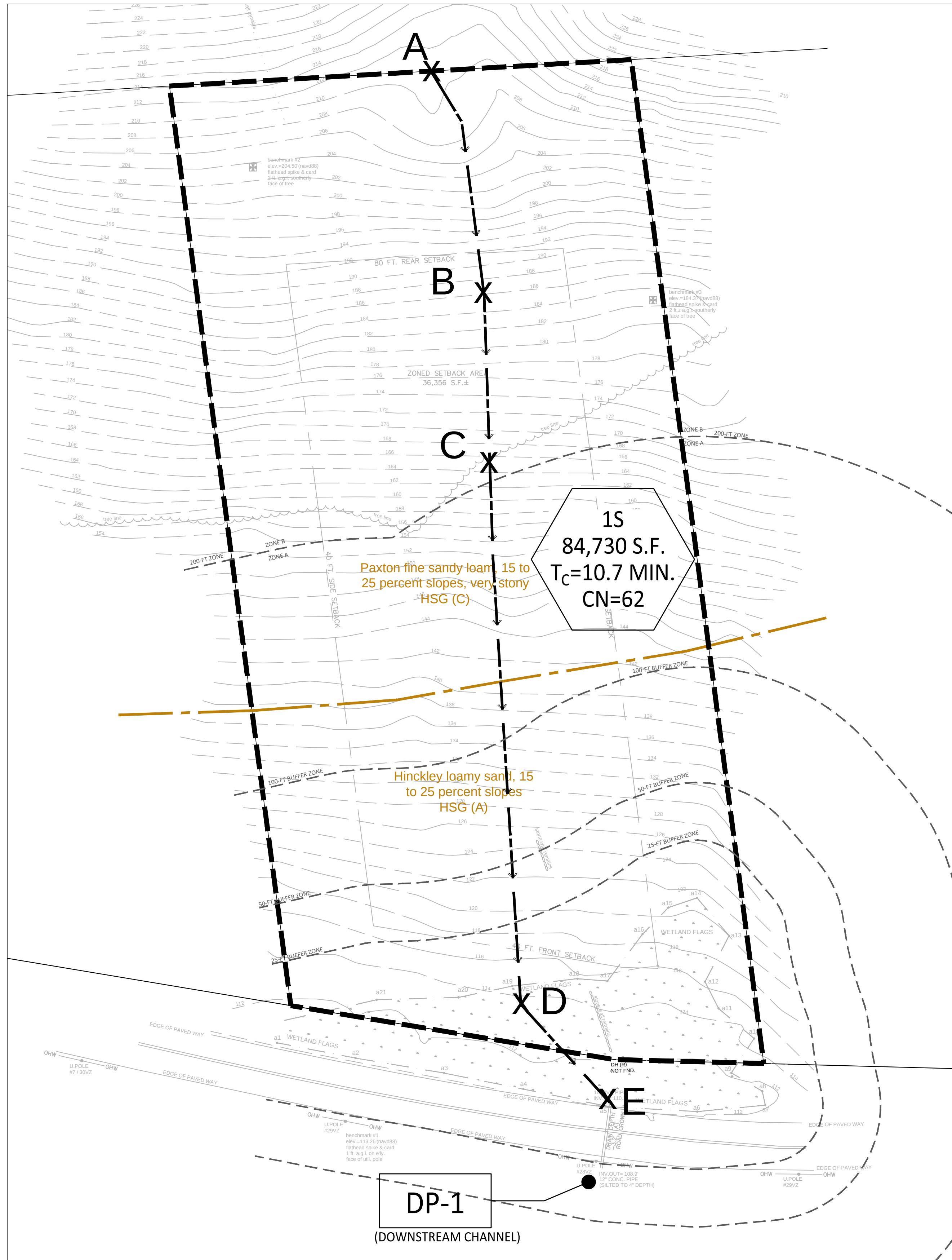
EXISTING CONDITIONS - DRAINAGE AREA MAP
