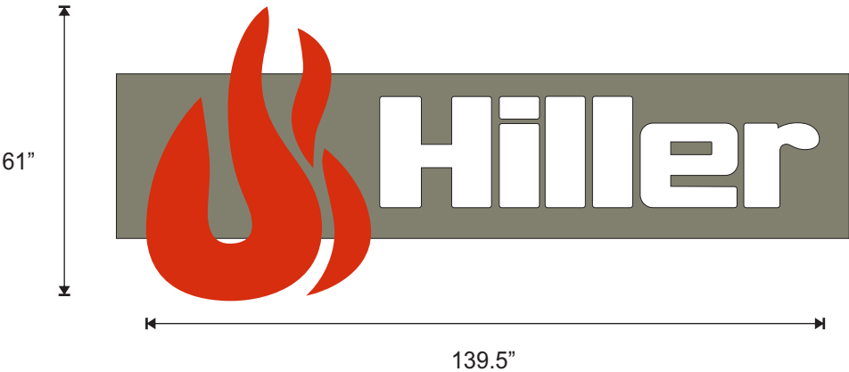
Standard duranodic bronze pan. Letters mount to face.
