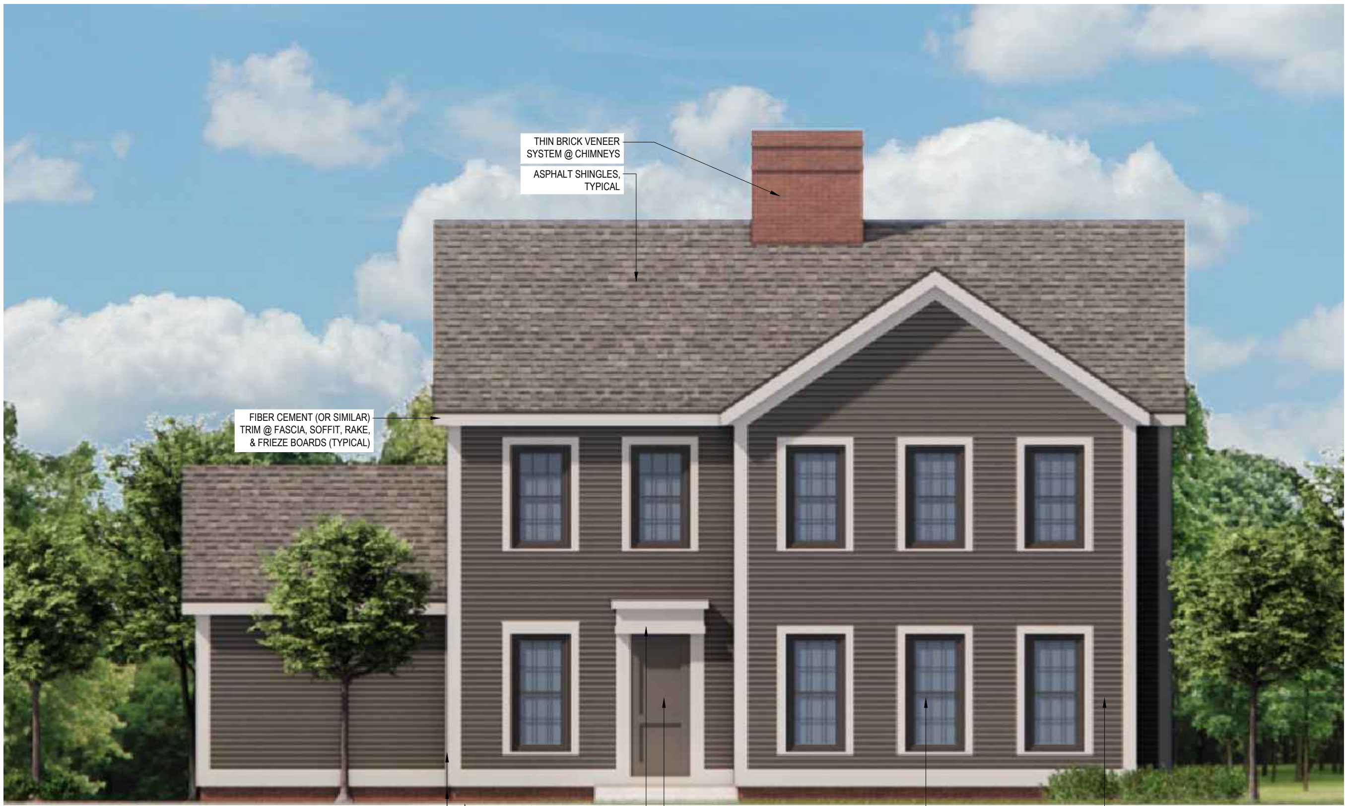
2 BUILDING A - SOUTH-EAST ELEVATION SCALE: 3/32" = 1'-0"
