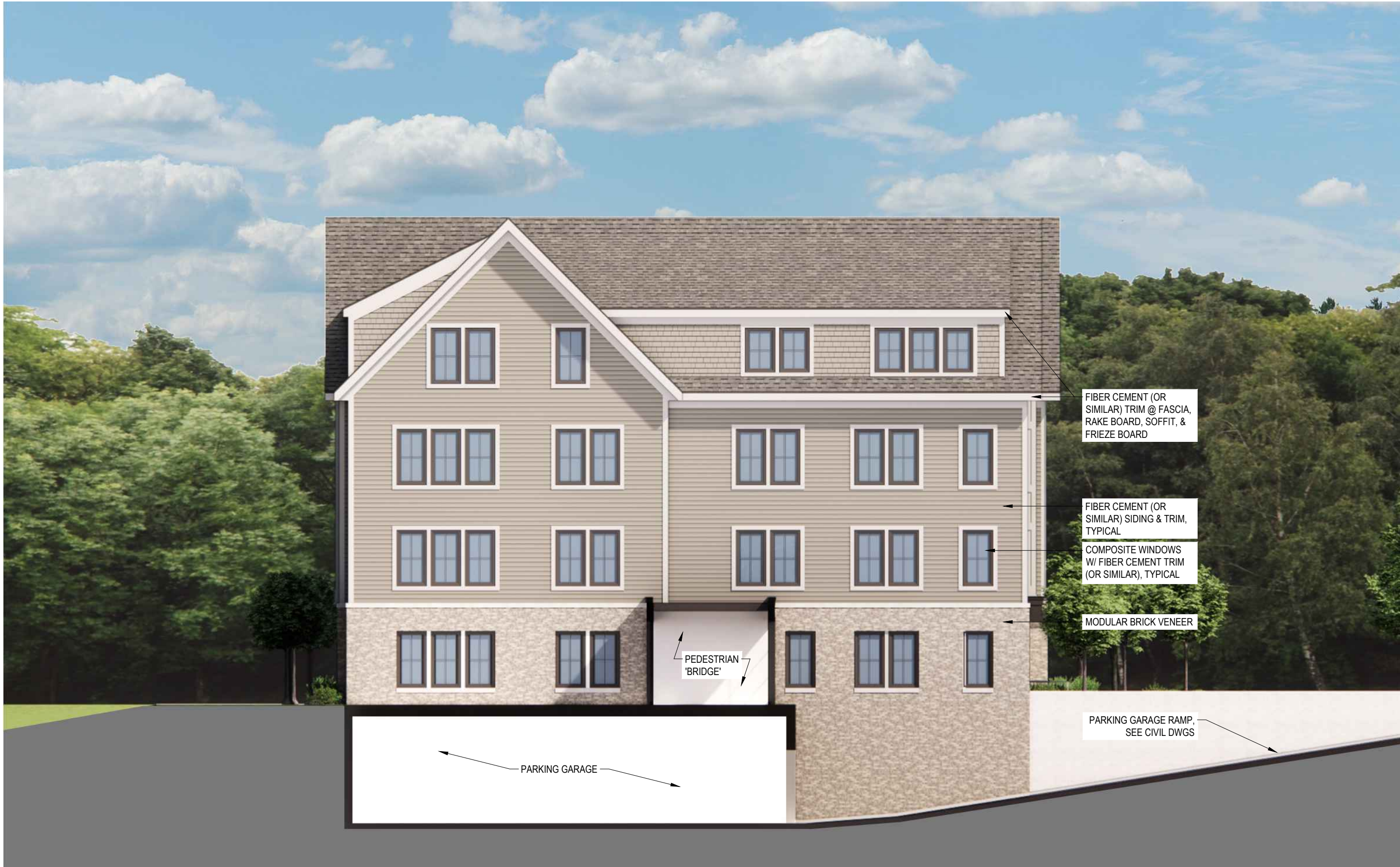
2 BUILDING C1 - SOUTH-EAST ELEVATION SCALE: 3/32" = 1'-0"
