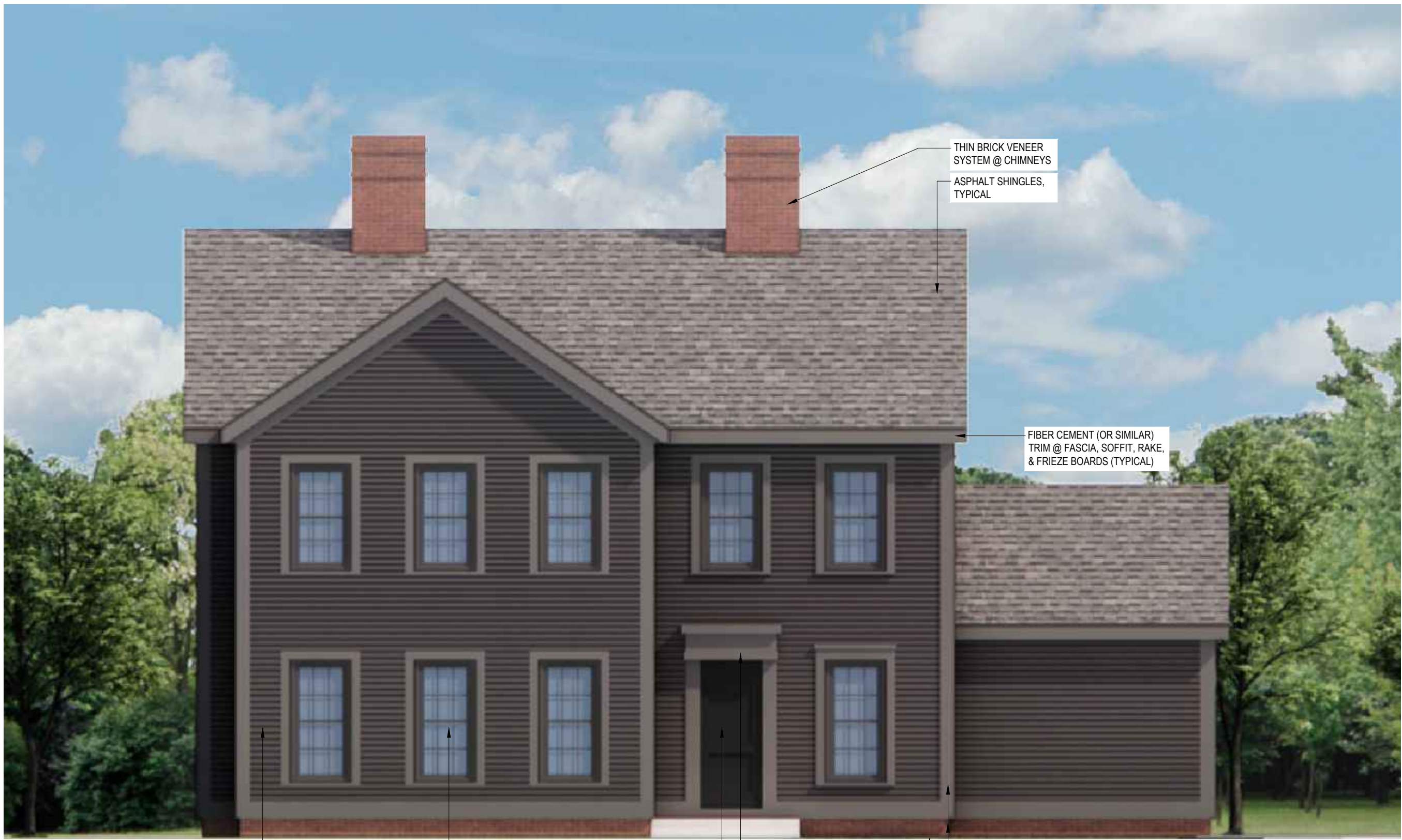
2 BUILDING B - SOUTH-EAST ELEVATION SCALE: 3/32" = 1'-0"
