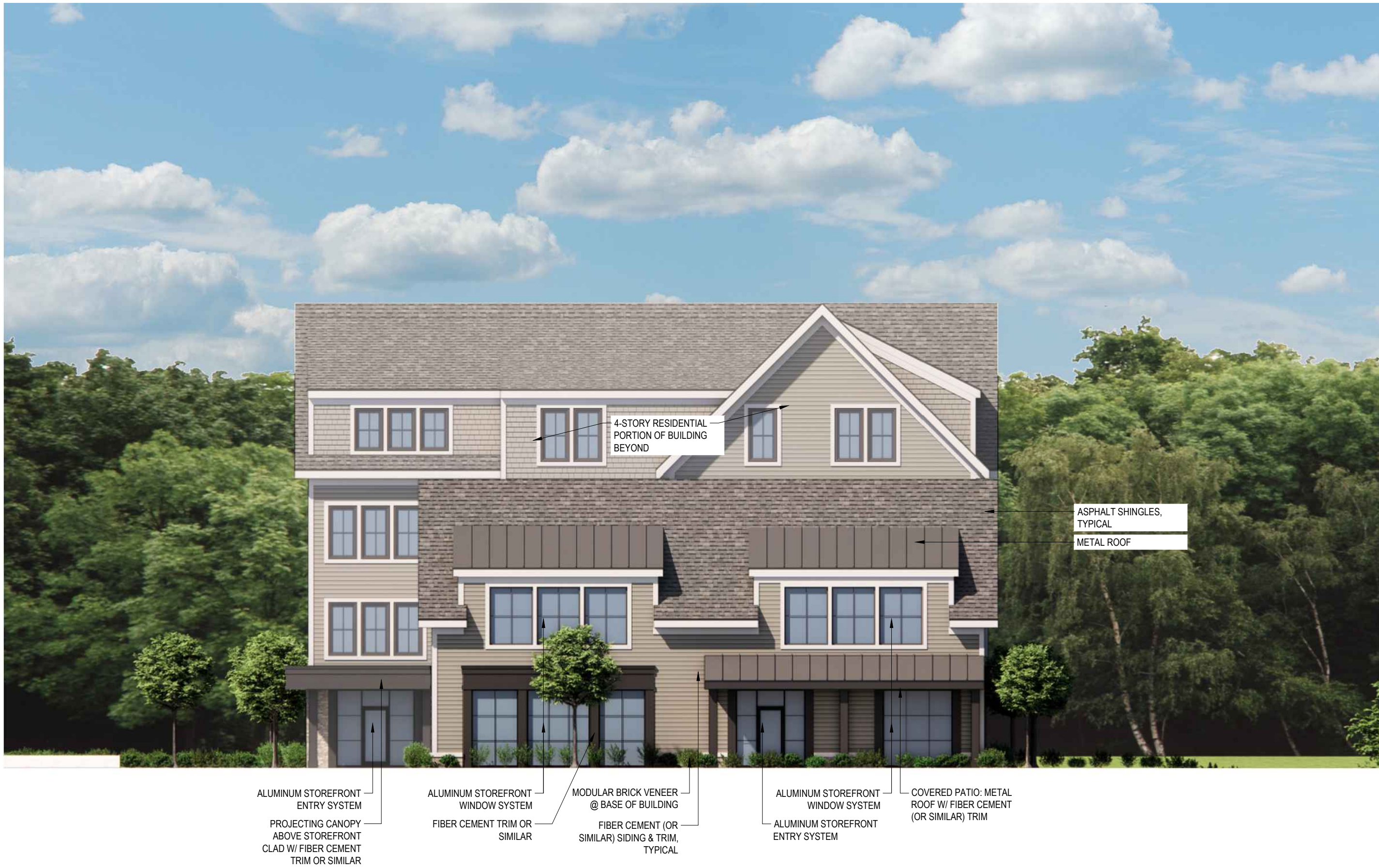
1 BUILDING C1 - NORTH-WEST ELEVATION SCALE: 3/32" = 1'-0"
