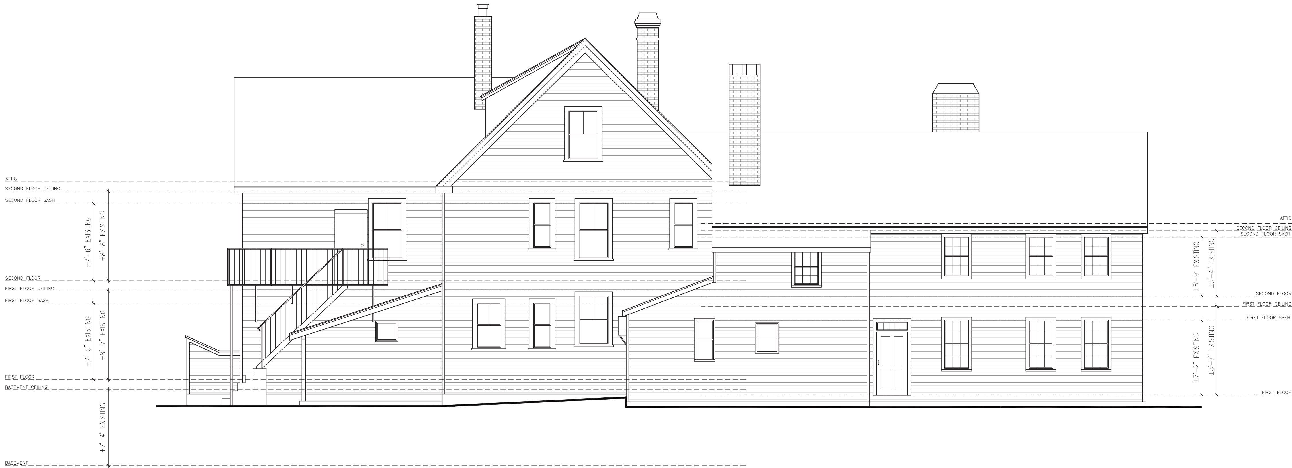
BUILDING D EXISTING LEFT ELEVATION SCALE: 3/16" = 1'-0"
